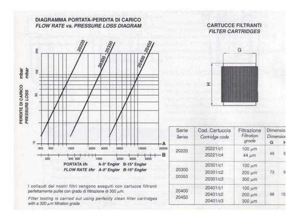
Filter testing is carried out using perfectly clean filter cartridges with a 300  $\mu$ m filtration grade.
